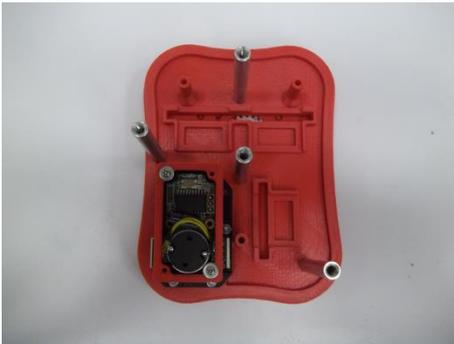
**IMPORTANT:** You should power up the Dynamixel with gear and drive it to its zero position. The arrangement of gears described in the previous page corresponds to the zero position of the geared Dynamixel. You can do this later during the final assembly steps, but it's easiest if you do it here.
