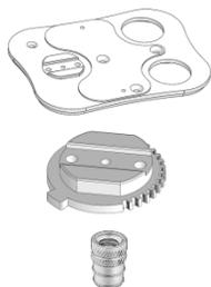
Install the remaining heat-set inserts in the finger base parts: *a1\_o.stl*, *c2\_left\_o.stl*, *c2\_right\_o.stl*. Note that *c2\_left\_o.stl* and *c2\_right\_o.stl* are mirrors of each other, so they are not interchangeable.
