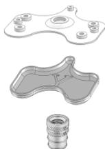
The palm pad is option, but it's a nice feature to have. Before pouring the mold, install the heated-inserts onto *d3\_base\_o.stl*. To cast the palm, tape the two mold halves together and place is such that *d3\_base\_o.stl* is on top. Pour the Vytaflex through the openings, enough so that the urethane is just short of filling up to the top surface.
