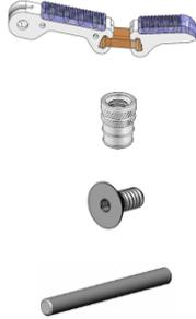
Press fit the 1/8" dowel pins for tendon-rerouting into the proximal link and back of the fingers. Use a soldering iron to install the heat-set insert into the distal link. The heat-set insert can be skipped in favor of using a nut for tendon termination.
